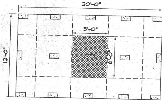
Note: Tributary area of shaded section on free standing deck shown is 5' x 6' = 30 sq. ft. Code will require a minimum footer of 8" x 16" per Table AM102.1.
