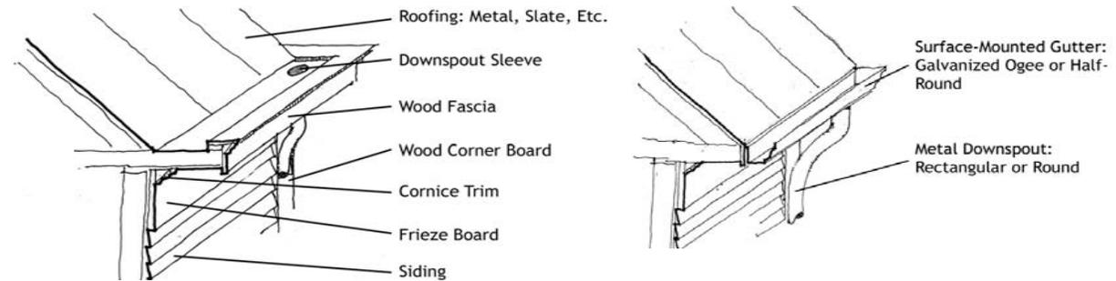
*hidden gutters (on left) and surface gutters (on right)*
